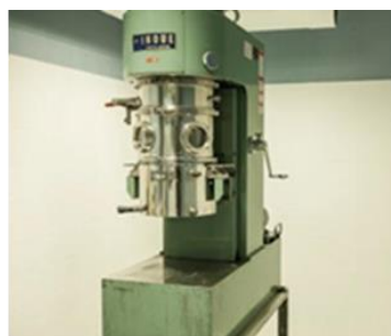
15 L mixer (for cathode slurry fabrication)
